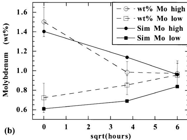
Fig. 6—Experimental and DICTRA simulated maximum/minimum dendrite compositions for AerMet100 as a function of homogenization time at 1173 °C for (a) chromium and (b) molybdenum.
