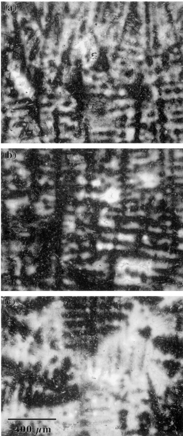
Fig. 4—Optical micrographs of the as-cast AerMet100 dendritic structure at the (a) ingot edge, (b) ingot midpoint, and (c) central core region.
