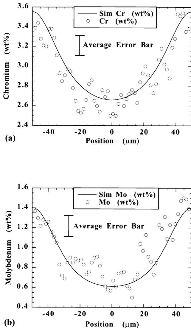
Fig. 5—Experimental and DICTRA simulated line profile compositions for as-cast AerMet100 across a 100- $\mu\text{m}$  secondary dendrite arm for (a) chromium and (b) molybdenum.
