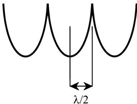
Fig. 3—Secondary dendrite arm spacing.
