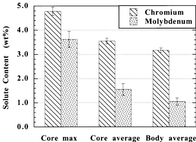
Fig. 7—Macroseggregation of chromium and molybdenum to the central core of the cast ingot.
