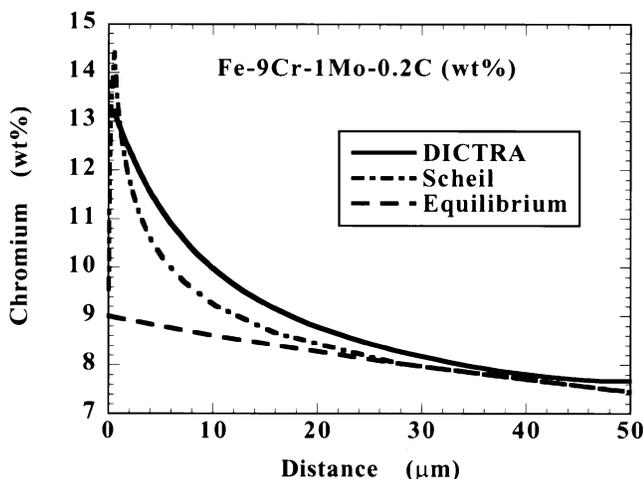
Fig. 2—Comparison of simulation models for chromium composition as a function of space in a 100- $\mu\text{m}$  secondary dendrite arm for the alloy Fe-9Cr-1Mo-0.2C (wt pct).
