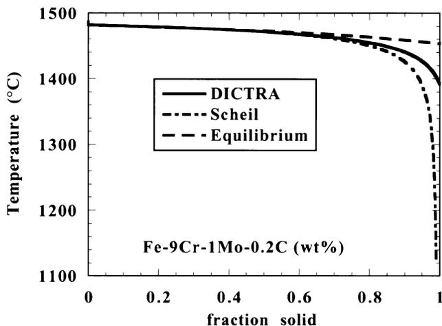
Fig. 1—Comparison of simulation models for the fraction solid as a function of temperature for the alloy Fe-9Cr-1Mo-0.2C (wt pct).
