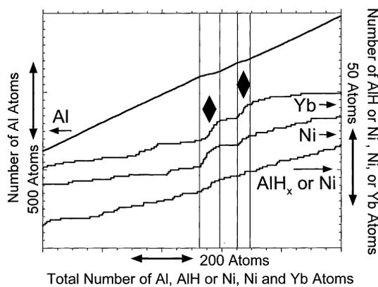
Fig. 6. Yb–Ni co-clusters (◆) in a multicomponent integral concentration profile for Al, Yb, Ni, and AlH<sub>x</sub> or Ni of melt-spun Al–5.2at.% Ni–6.8at.% Yb heated to 188 °C at a rate of 10 °C min<sup>-1</sup>. The clusters can safely be recognized, in spite of a convolution of the Ni<sup>+</sup>-peaks in the mass spectrum by the formation of AlH<sub>x</sub><sup>+</sup> complex ions during pulsed field evaporation.
