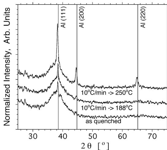
Fig. 3. X-ray diffractograms of melt-spun Al–5.2at.% Ni–6.8at.% Yb in the as-quenched state and heated to 188 or 250 °C, respectively, at a rate of 10 °C min<sup>-1</sup>, employing Cu-K $\alpha$ -radiation. The intensities are normalized by the integral intensity of the respective first, dominant peak. The positions of the Bragg peaks of pure Al are marked by vertical lines.
