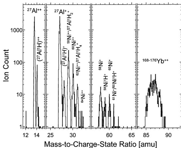
Fig. 1. Atom-probe time-of-flight mass spectrum of an Al–5.2at.% Ni–6.8at.% Yb alloy heated isochronally to  $188 \text{ }^\circ\text{C}$  at a rate of  $10 \text{ }^\circ\text{C min}^{-1}$ .
