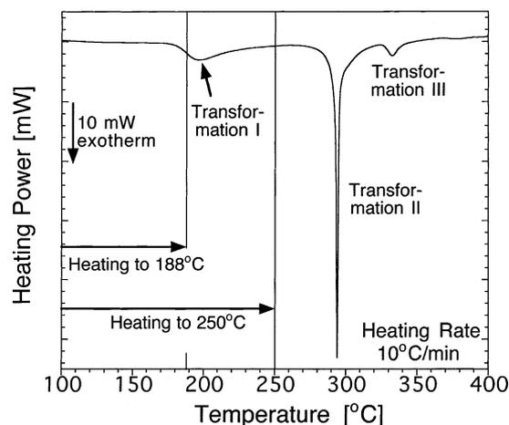
Fig. 2. Differential scanning calorimetry thermogram of melt-spun Al–5.2at.% Ni–6.8at.% Yb. The heating rate is  $10 \text{ }^\circ\text{C min}^{-1}$ . The transformation stages investigated in this study, at the beginning of transformation I and with transformation I completed, are indicated.
