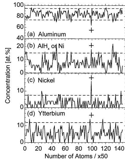
Fig. 4. Ni-rich cluster (+) in an atom-probe concentration profile of melt-spun Al–5.2at.% Ni–6.8at.% Yb in the as-quenched state. The horizontal dashed lines in each concentration profile are the two-sigma limits of a random concentration distribution with the same average composition and block size, encompassing an average 96% of the measured values. Concentration peaks distinctively exceeding the dashed lines are significant.
