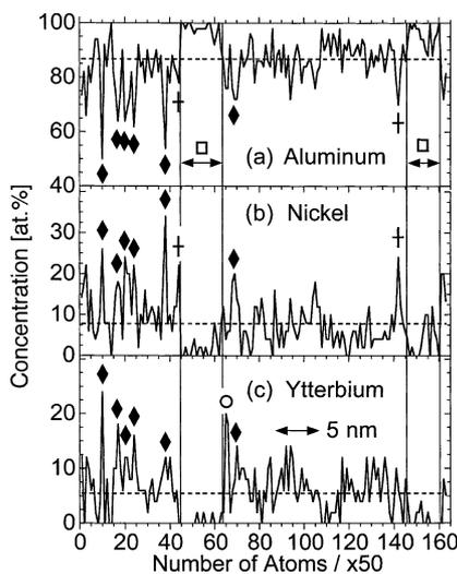
Fig. 7. Yb–Ni co-clusters (◆), Ni-rich clusters (+), and Yb-cluster (○) in a multicomponent atom-probe concentration profile of melt-spun Al–5.2at.% Ni–6.8at.% Yb heated to 250 °C at a rate of 10 °C min<sup>-1</sup>. The horizontal dashed lines are the concentrations averaged over the entire profile.
