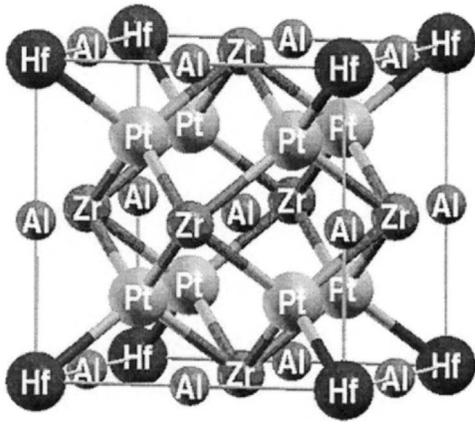
FIG. 1. Atomic structures of the mixed phase,  $\text{Pt}_2(\text{Hf}_{0.75}\text{Zr}_{0.25})\text{Al}$ . Note that the replacement of Hf with Zr generates the  $L_{21}$  Heusler alloy of  $\text{Pt}_2\text{ZrAl}$ .
