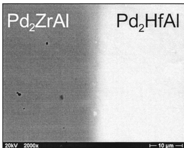
FIG. 2. BSE image of a cross section of the Pd<sub>2</sub>HfAl/Pd<sub>2</sub>ZrAl diffusion couple annealed at 1100 °C for 50 h.
