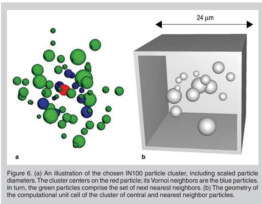
Figure 6. (a) An illustration of the chosen IN100 particle cluster, including scaled particle diameters. The cluster centers on the red particle; its Voronoi neighbors are the blue particles. In turn, the green particles comprise the set of next nearest neighbors. (b) The geometry of the computational unit cell of the cluster of central and nearest neighbor particles.
