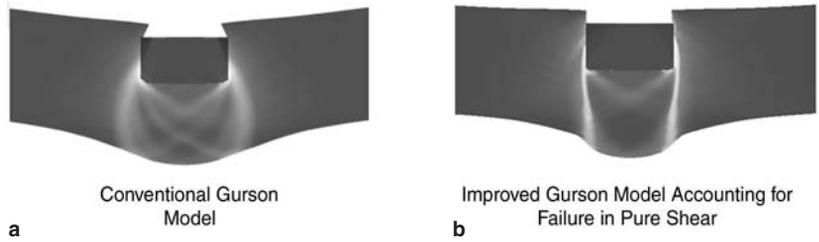
Figure 8. The contours of equivalent plastic strain are plotted for the solution given by (a) the conventional Gurson model and (b) for the improved Gurson, accounting for the microvoid softening failure mechanisms in pure shear. The improved model displays the plugging effect observed experimentally.<sup>21</sup>
