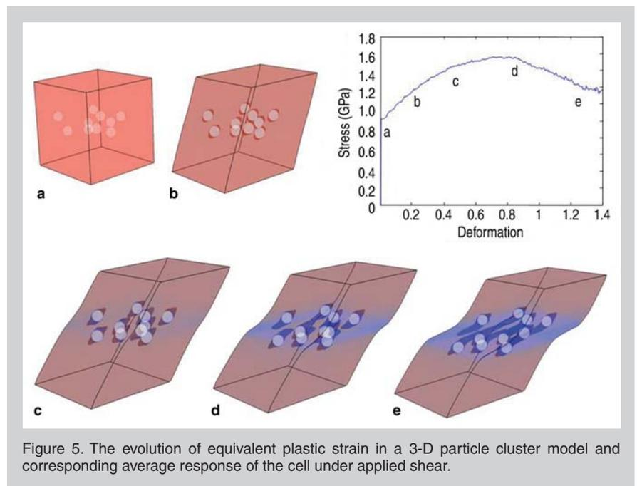
Figure 5. The evolution of equivalent plastic strain in a 3-D particle cluster model and corresponding average response of the cell under applied shear.
