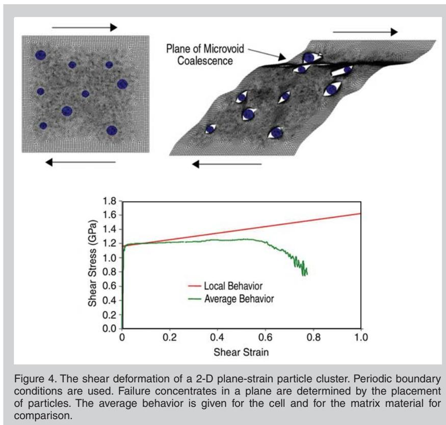
Figure 4. The shear deformation of a 2-D plane-strain particle cluster. Periodic boundary conditions are used. Failure concentrates in a plane as determined by the placement of particles. The average behavior is given for the cell and for the matrix material for comparison.
