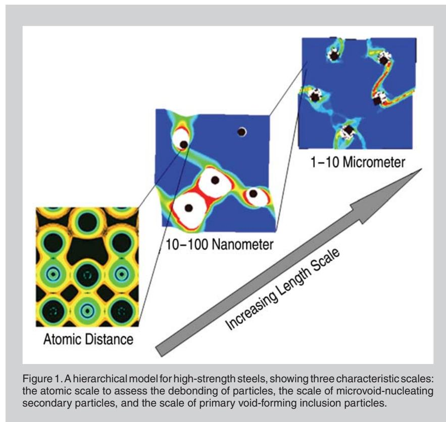
Figure 1. A hierarchical model for high-strength steels, showing three characteristic scales: the atomic scale to assess the debonding of particles, the scale of microvoid-nucleating secondary particles, and the scale of primary void-forming inclusion particles.
