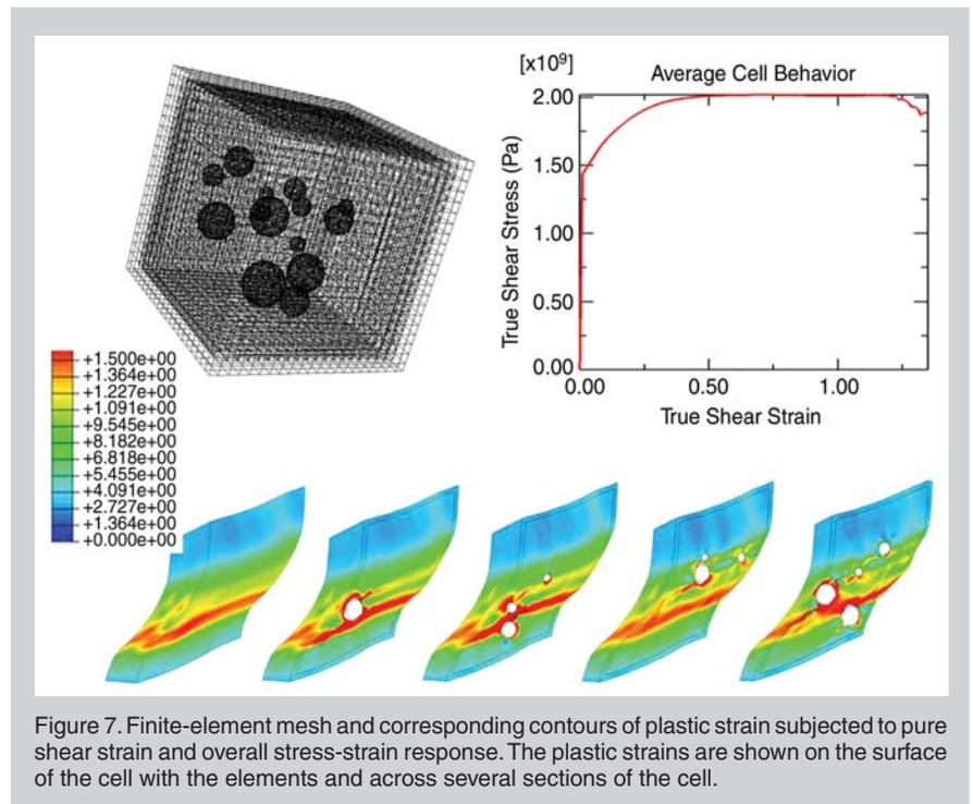
Figure 7. Finite-element mesh and corresponding contours of plastic strain subjected to pure shear strain and overall stress-strain response. The plastic strains are shown on the surface of the cell with the elements and across several sections of the cell.
