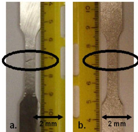
Figure 6. a) Demonstration of a pre-healed composite with a through matrix crack. b) Demonstration of a healed composite.
