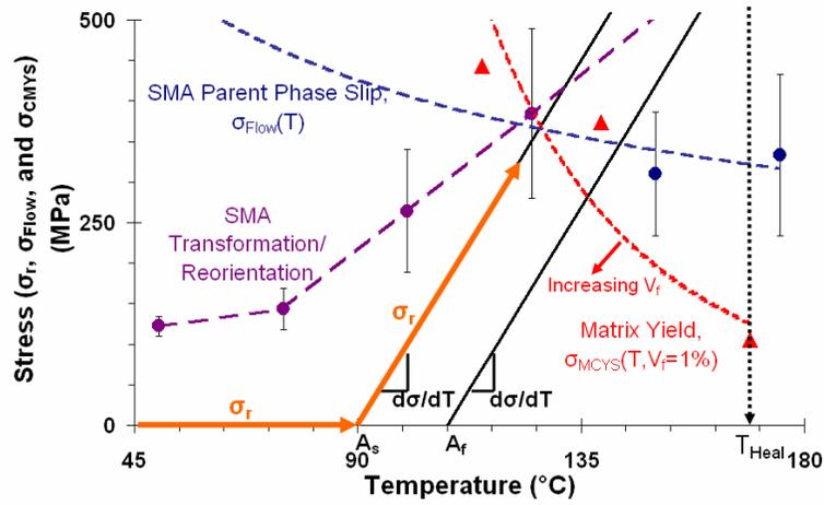
Figure 4. Stress versus temperature plot illustrating the evolution of reversion stress in the SMA wire as a function of temperature.
