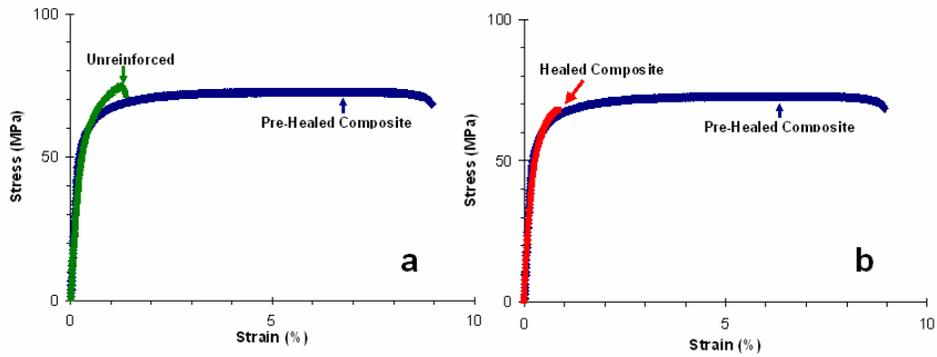
Figure 5. a) Comparison of stress-strain curves of the unreinforced matrix alloy and SMA reinforced composite ( $V_f=1\%$ ). b) Comparison of typical stress-strain curves of an pre-healed ( $V_f=1\%$ ) and healed composite ( $V_f=1\%$ ).
