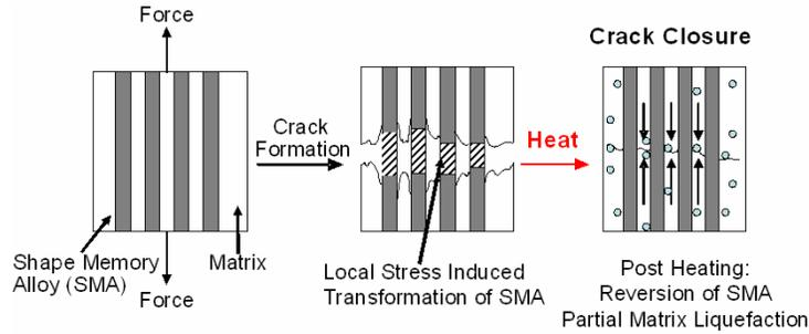
Figure 1. Schematic overview of the self-healing process
