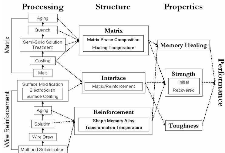
Figure 2. Self-healing alloy composite systems design chart.
