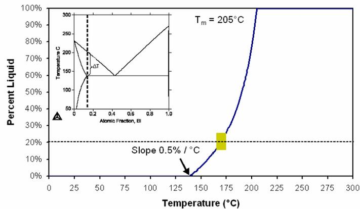
Figure 3. Phase diagram of the Sn-Bi alloy system indicating the composition used for the matrix and the fraction of liquid versus temperature curve displaying gradual melting behavior at healing temperature of 169°C.
