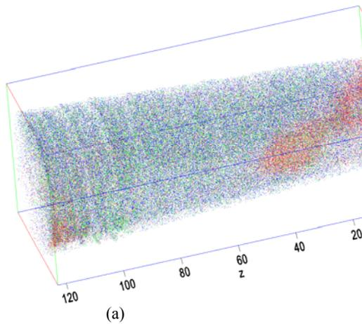
Fig. 2. (a) LEAP tomographic reconstructions of Mg-7Zn-3Al using the voltage-pulse mode;
