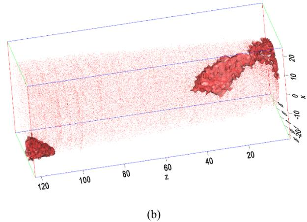
Fig. 2. (b) LEAP tomographic reconstructions of 20 % Zn isoconcentration surfaces;
