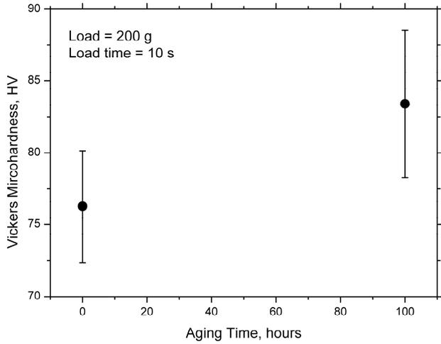
Fig. 1. Vickers microhardness vs. aging time at 150 °C for Mg-7Zn-3Al. Error bars are one standard deviation from the average.
