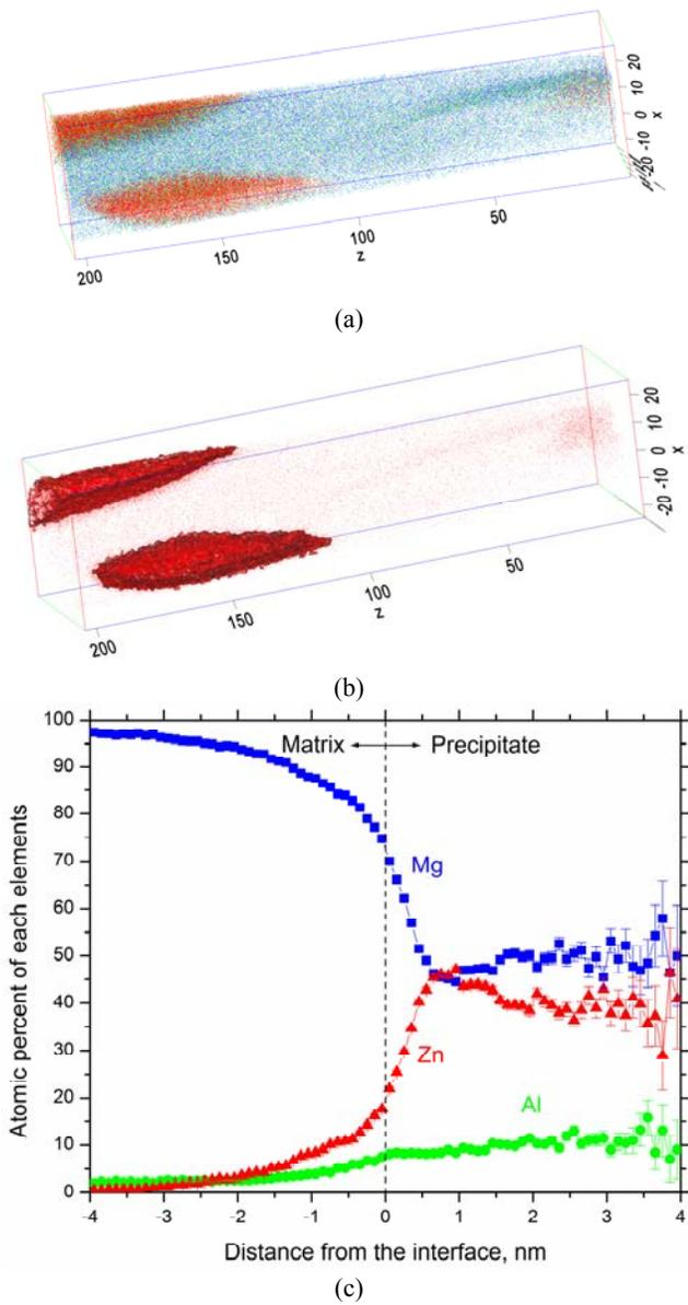
Fig. 3. (a) LEAP tomographic reconstructions of Mg-7Zn-3Al using the laser-pulse mode; (b) LEAP tomographic reconstructions of 20 % Zn isoconcentration surfaces; (c) Proximity histogram for the LEAP tomographic reconstructions displayed in Fig. 3 (a) showing the average concentration of Mg, Al and Zn as a function of distance from the Mg-Zn-Al ternary heterophase interfacial, as defined by a 20 at. % Zn isoconcentration surface.
