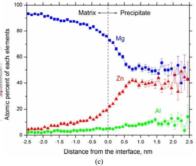
Fig. 2. (c) Proximity histogram for the LEAP tomographic reconstructions displayed in Fig. 2 (a) showing the average concentration of Mg, Al, Zn and Ca as a function of distance from the Mg-Zn-Al ternary heterophase interfacial, as defined by a 20 at. % Zn isoconcentration surface.
